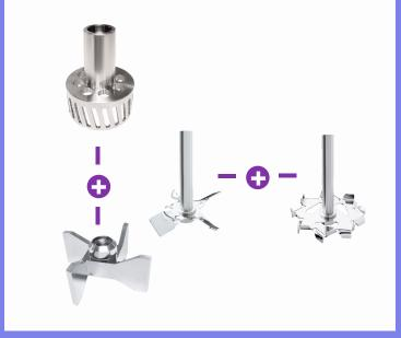
The Starter and Master Lab Packages are available in 6 references, varying according to the dimensions of the tools, adapted to the volume of the beaker to guarantee a homogeneous mixing (references for a volume of 250, 600, 1000, 2000, 3000 or 5000 mL). The Turbotest® shaft with tool and its attachment system allow an easy and quick shaft changing.
