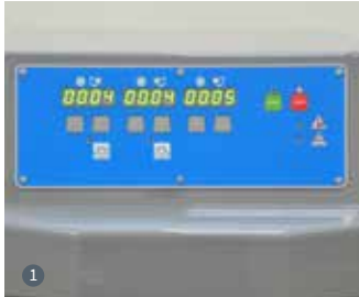
1 Electronic control panel to programme 20 recipes
